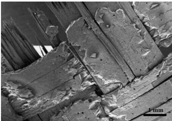
Fig. 10. Epoxy surface on tensile bar subjected to 2.0 MGy gamma radiation.
